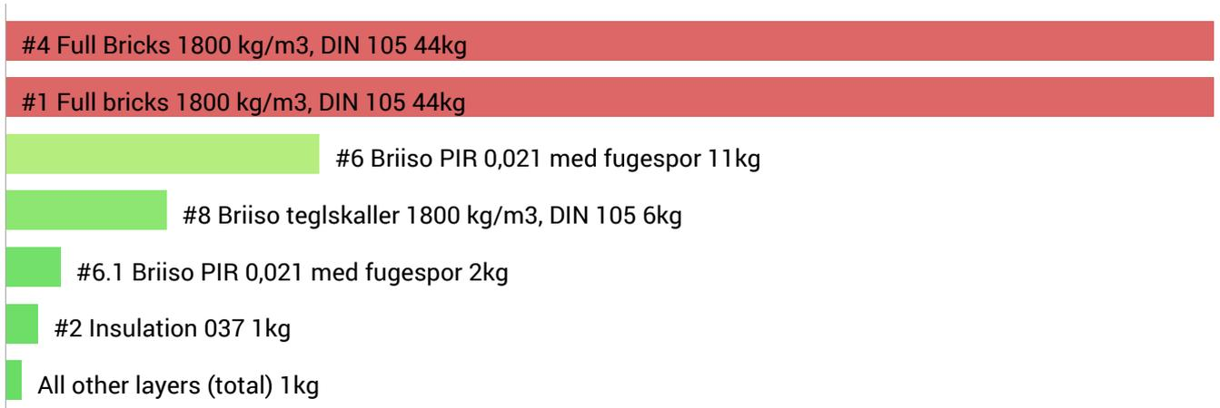
254 mm facade with insulated cavity + 32 mm PIR,  $U=0,30 \text{ W}/(\text{m}^2\text{K})$
