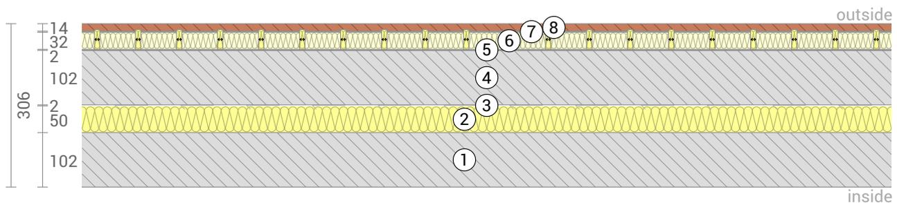
254 mm facade with insulated cavity + 32 mm PIR, U=0,30 W/(m²K)
