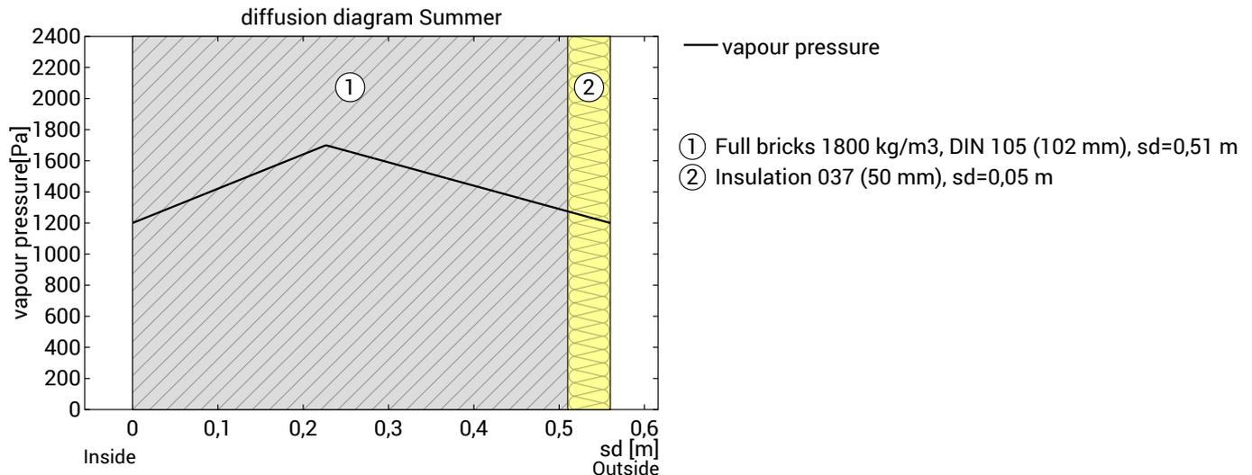
Condensate-free component: The maximum possible evaporation mass for the drying reserve is calculated. Consider the level that has the lowest evaporation potential in the dew period, at sd=0,23 m, within layer Full bricks 1800 kg/m<sup>3</sup>, DIN 105:
